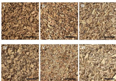
Fig. 1: Overview of the substrates used in this study. Douglas fir ( Pm ) bark (I), Scots pine ( Ps ) bark (II), and European birch ( Bp ) bark (III). 50:50 ratio mixtures: Douglas fir bark with beech wood ( Fs ) (IV), pine bark with beech wood (V), and birch bark with beech wood (VI). Scale bars represent 10 mm.
